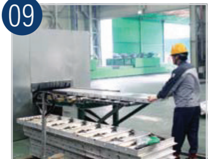
Leveling & adjustment of panels
